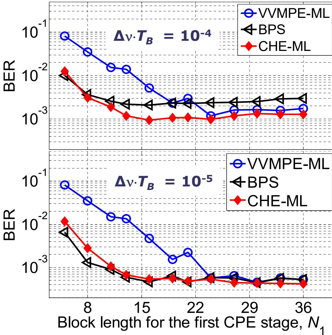
When phase noise increases ( $10^{-5} \rightarrow 10^{-4}$ ), the linewidth tolerance is slightly degraded for BPS compared to VVMPE-ML and CHE-ML
