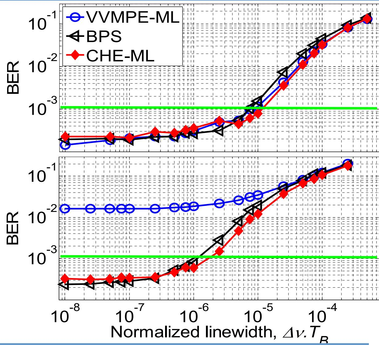
Maximum tolerated linewidths of 520 and 70 kHz for 40 Gbaud
