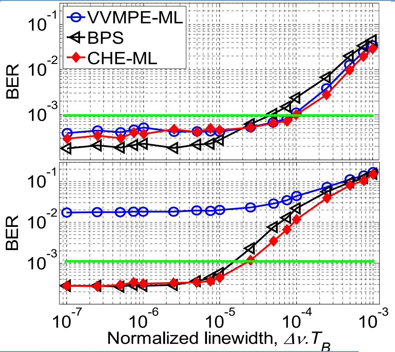
Maximum tolerated linewidths of 1 MHz and 680 kHz for 40 Gbaud
